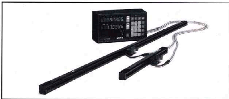
Sony Precision programmable digital read out with lathe package attached. (Photo courtesy of Antarra Communications.)
